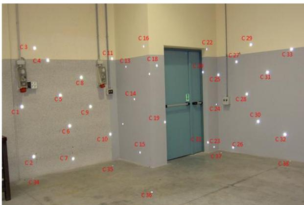
Figure 1. The calibration test-field
