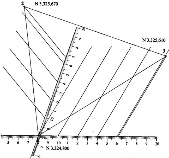
**Fig. 5.** Establishing 200 m northing intervals on original triangle
