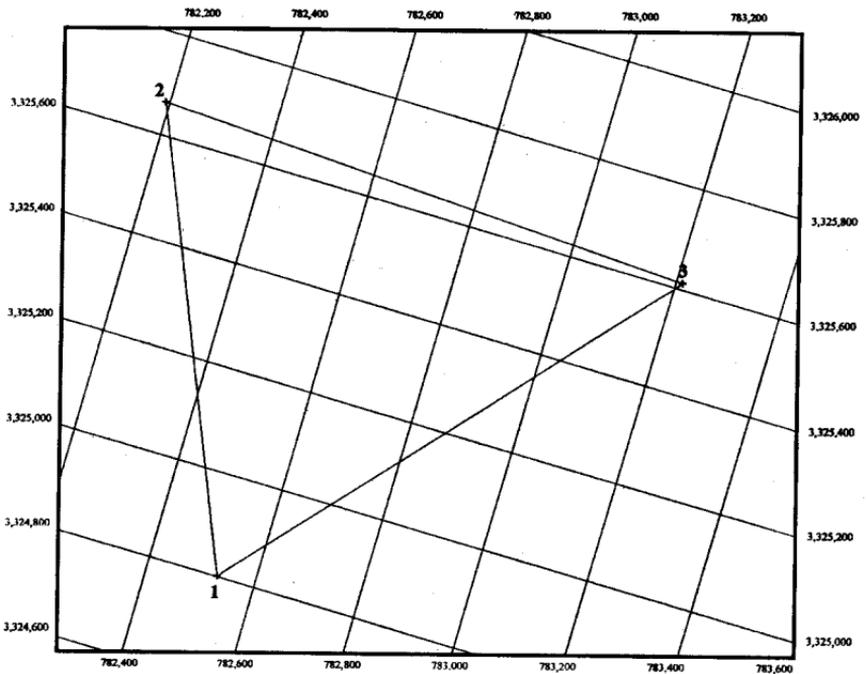
**Fig. 7.** Combining easting and northing lines to form 200 m grid
