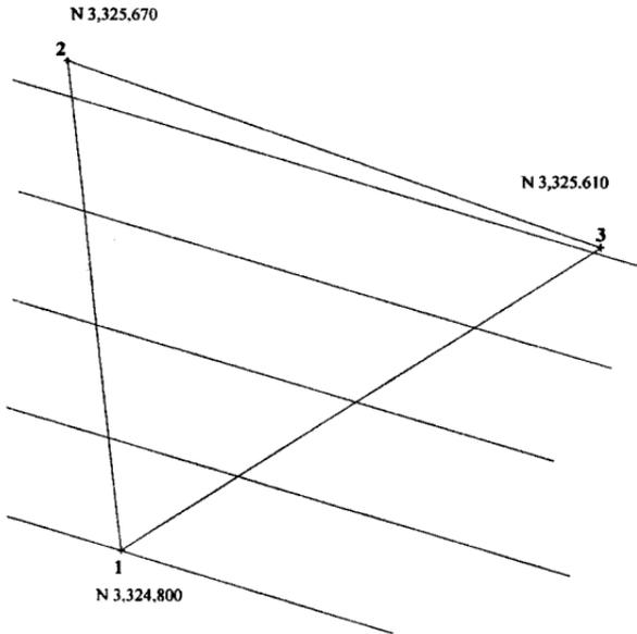
**Fig. 6.** Triangle with established northing lines
