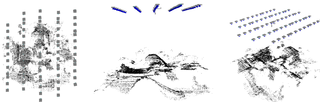
Fig. 4. Automatic orientation results for the UAV block over Copan (Honduras): 3D points and camera poses.
