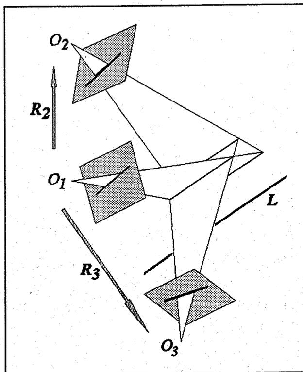
**Figure 11:** Basic geometry of (rotational) relative orientation of image triples using straight lines. The three homologous projective planes intersect in the model line  $L$ .
