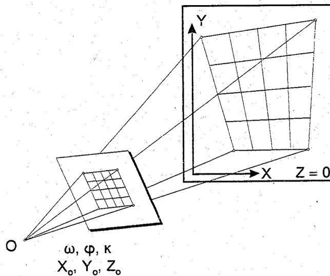
**Figure 20:** A synthetic regular grid of 72 image points have been projected back to the object assuming known e.o.
