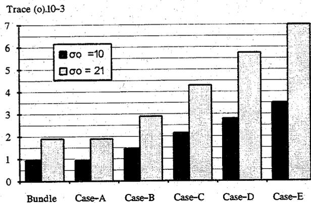
Figure 7: trΣ in all tested cases in comparison to that of regular bundle with point measurements.
