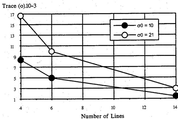
**Figure 6:** Values of  $\text{tr}\Sigma$  for different number of control lines (see Fig. 5) and different level of measurement noise for Case-B.
