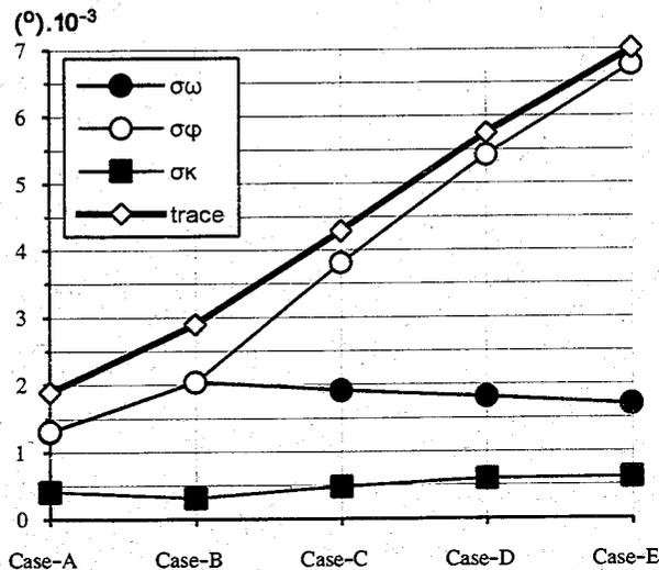
**Figure 9:** RMS values for the rotation angles and the  $\text{tr}\Sigma$  for all tested cases for measurement noise of  $\sigma_0=21\mu\text{m}$  level.
