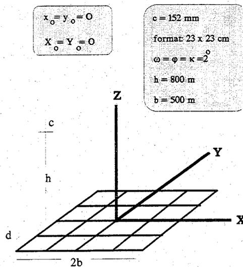
**Figure 2:** The simulated grid of points and the used ground coordinate system.
