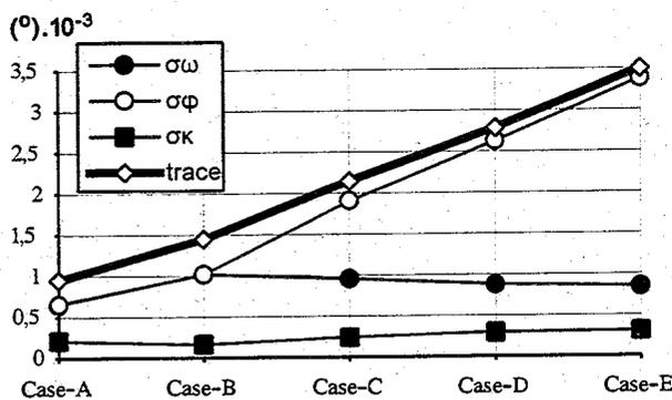
Figure 8: RMS values for the rotation angles and the trΣ for all tested cases for measurement noise of  $\sigma_0 = 10\mu\text{m}$  level.
