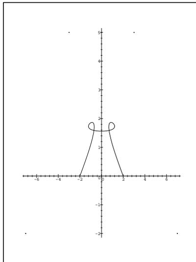
Figure 3.1: A  $6^{\text{th}}$  degree Bézier curve.
