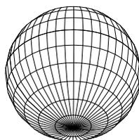
Figure 2.2: An example of a non-developable surface.
